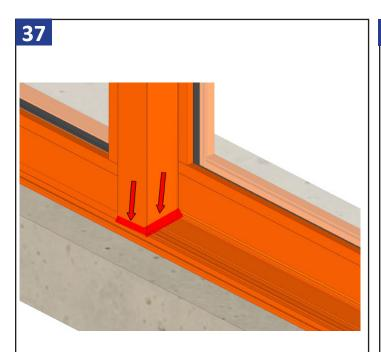
Silicone along the bottom of the exterior of the interlock.
