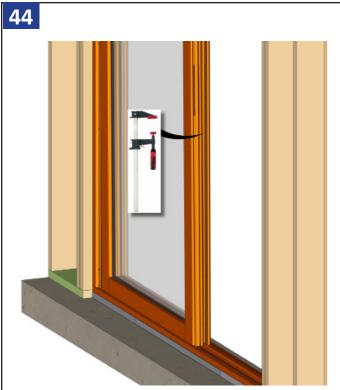
After the rollers are adjusted, open the door, and place a clamp on the active jamb to the fixed jamb holding the active panel in place so it cannot fall out.
