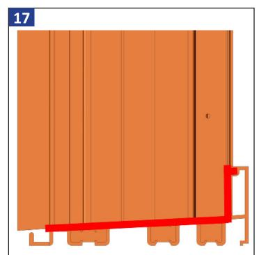
Apply silicone to seal the back of the frame and sill connection, then tool in.
