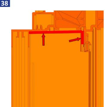
Press fixed panel weep baffle (Part #: QWP-50x75X60) in above the top of the fixed panel between the panel and frame. Then silicone and tool in smoothly with a putty knife.
