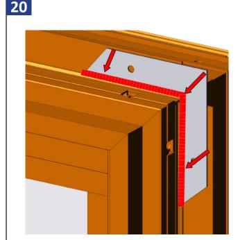
Remove backing off of the nail fin corner and attach the nail fin corner to the nail fins. Then silicone along the frame as shown above.
