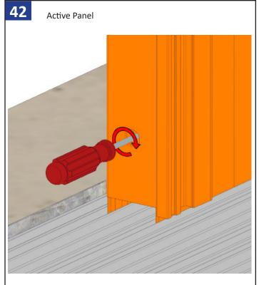
Use a #2 phillips screwdriver to engage the roller adjustment, on both sides of a panel. Adjust the rollers about half way up, this will help you align the roller on the track properly.
