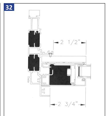
See above diagram. Be sure the fixed panel is seated fully into the frame jamb.
