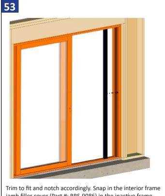
jamb filler cover (Part #: BRS-9086) in the inactive frame
