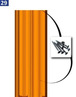
Fully fasten the screws down now to hold the frame in place. The holes through the interior track of the header & jambs, typically 6" from ends and 24" on center for fasteners. All fastener locations are to shimmed between framing and condition.
