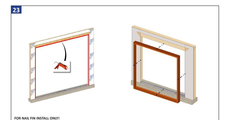
frame by sliding in the rough opening with the fin to the exterior side. Set frame onto the sill pan.
