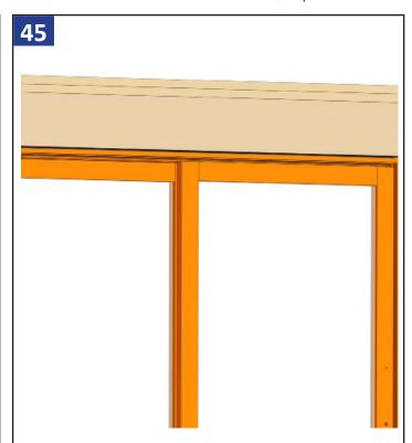
Take the head closure, trim to fit between the jamb closures, and slide it over the head of the panel.
