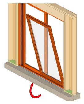
On the interior side set the active panel on the roller track. Make sure the panels are overlapped when installing so the interlocks will engage properly. Slide panel to the fixed jamb. Make sure the closure captures active panel and operates properly.
