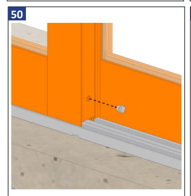
Once all panels have been adjusted install the panel bumpers into each roller adjustment hole.
