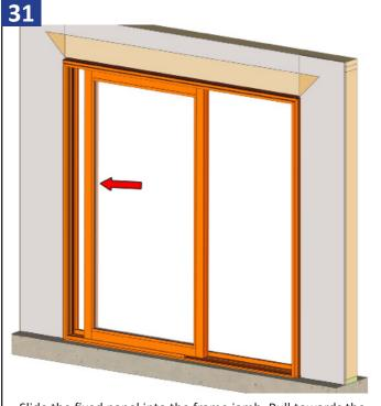
Slide the fixed panel into the frame jamb. Pull towards the exterior this will help in the next steps.
