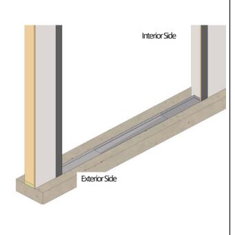
Rough fit the sill pan in place to ensure of proper fitment.
