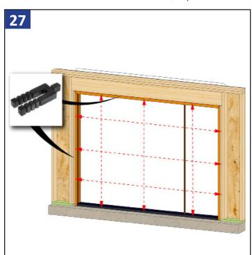
Check that the door frame is not bowed at jambs or head, a string line may be required. Adjust shims as needed but verify measurements are within 1/16".
