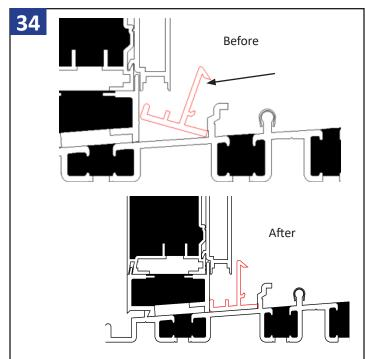
Lock the panel sill in place with three sill compression locks (Part #: M25381-PCS). Set fixed panel sill compression lock down in the track and then take a flat head screw driver and pop into place as shown above.
