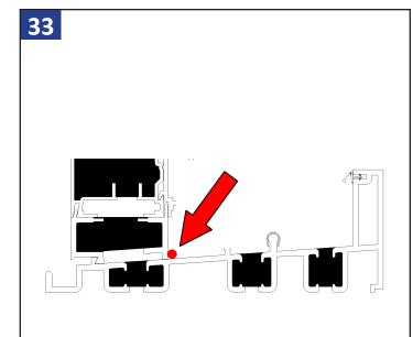
Run a bead of sealant along the base of the setting chair on the interior side.
