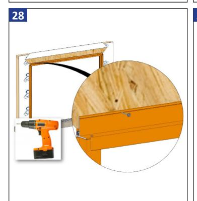
**NAIL FIN ONLY!**Fully tighten the fasteners down now to hold the frame in place. All fastener locations are to shimmed between framing and condition
