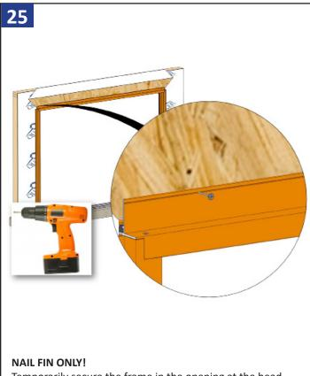
Temporarily secure the frame in the opening at the head corner(s) by tacking a fastener through a slotted hole in the nail fin.
