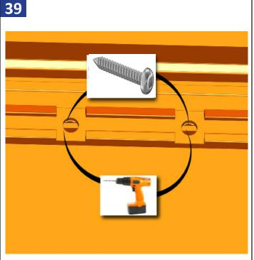
To secure the fixed panel, drill a 11/64" hole into the panel along the frame where the holes are already pre drilled. Holes will be along the frame jamb, and there will also be 2 in the frame head.
