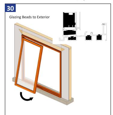
From the exterior, install the fixed panel with the setting chair, by tilting the top into the exterior most head track. Set the bottom of the fixed chair against the lip of the sill.
