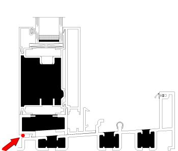
On the exterior side, run a continuous bead of sealant along the bottom of the setting chair, (DO NOT COVER THE WEEPS).
