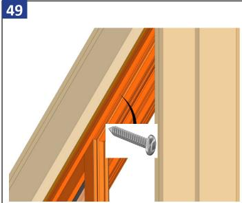
Slide the panel over to finish drilling and installing fasteners in the head closure.
