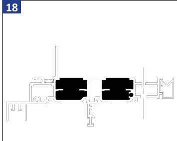
First drill a hole (11/32") through the frame, as shown above. Then take a 3/8" drill bit and drill through the first web making a clearance hole for the fasteners head clear. Install fasteners (Part #: MF#10-12X21/2).
