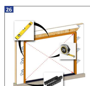
Square, level, and plumb the frame. Adjust shims as needed until diagonal measurements are within 1/8". Shim behind the header and jambs as necessary.
