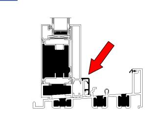
Measure from the interlock of the fixed panel to the front of the frame jamb and cut to length. Then snap the vinyl frame parting (Part #: BRS-9052) with a rubber mallet. Strip cover in the sill along the fixed panel that runs from frame jamb to panel meeting rail.
