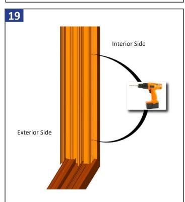
Drill holes through the frame of the header & jambs, typically 6" from ends and 24" on center. (Drill bit size is based off the fasteners size being used.)
