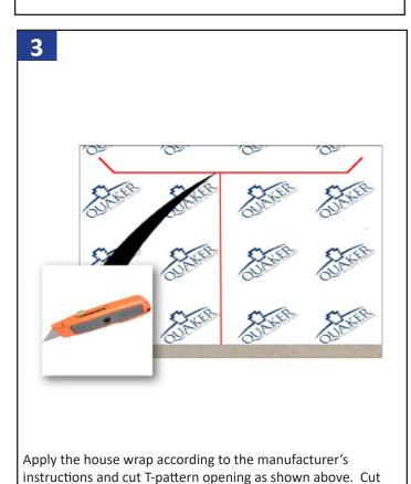
top flap angles at 45 degrees and 1" longer than the width of
