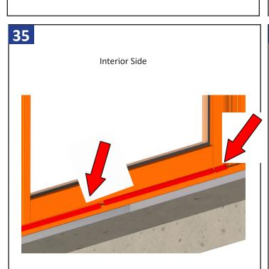
Take baffle(Part #: QWP-50x75X60), cut to length, then press the baffle down between compression locks and the frame. The baffle will run full length.
