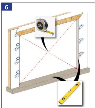
Check that the opening is square. The diagonal measurements need to be within 1/8" of each other. Verify the rough opening is plumb and level.
